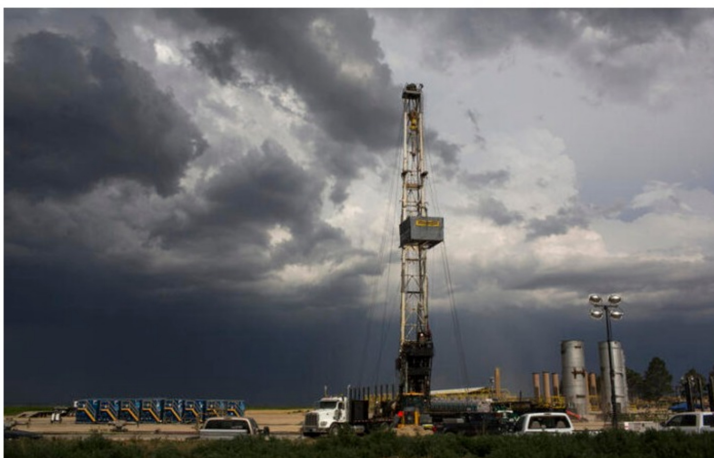
A hydraulic fracturing drilling rig creating a new well on the Niobara shale formation, one of the most intensively fracked areas in the United States.
